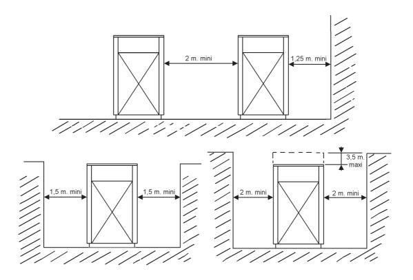
Unit dimensional drawings enable the optimum position of the units to be determined both for installation and maintenance
