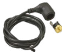
2075KIT01 Bimetallic safety button thermostat with M4 fixing screw. Operating temperature: 55°C. Contact flow rate (usually closed): 10A 250Vac. Comes with a connection cable.
