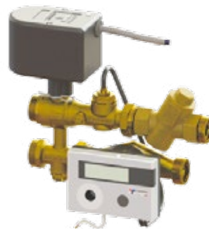
6502G03DYN "SHORTY DYNAMIC" metering module consisting of compact calorimeter counter, 3-way motorized zone valve for heating/cooling systems, PICV dynamic balancing valve.
