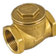
3665 Swing check valve FULL ISO228 female/female with brass shutter without gasket
