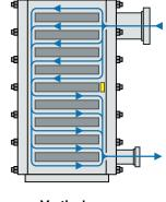
**Vertical** for Liquid-Liquid and Multipass Condensers and Evaporators
