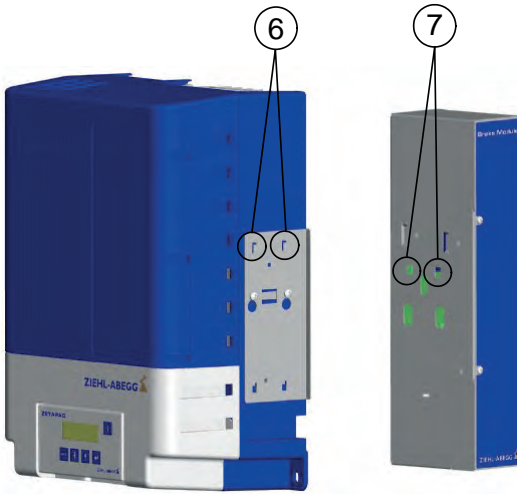
6 top hook of the fastening plate 7 openings of the Brake Module
