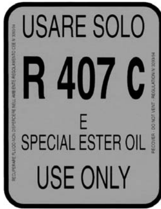
Identification of the refrigerant - External door
