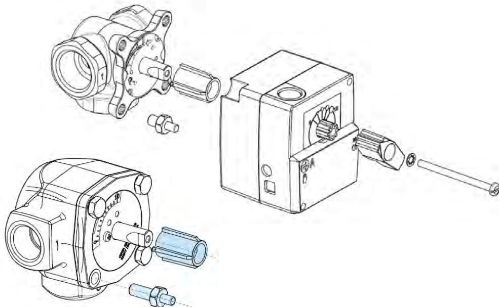
1. Check the rotation direction of the valve. By default the valve open clockwise.
