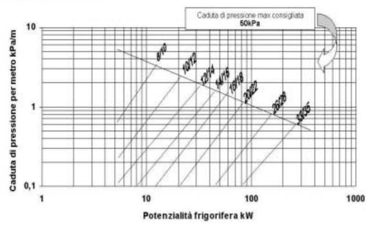
Figure 15: diagram for refrigerant pipeline dimensioning.
