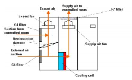
Figure 5: surgical room air conditioners without heat recovery
