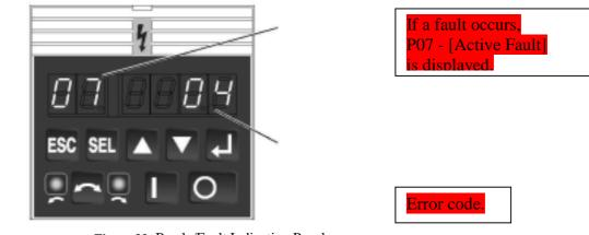
Figure 33: Ready/Fault Indicating Panel
