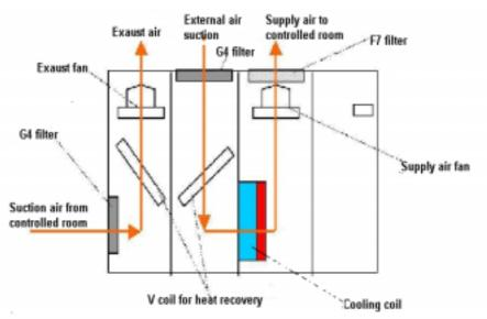
Figure 4: surgical rooms air conditioner with heat recovery
