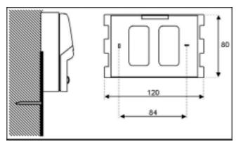
Figure 26: Wall-mounting of the user interface.
