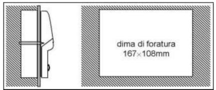
Figure 25: Panel-mounting of the user interface.
