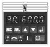
Figure 30: Program Keypad Module.
