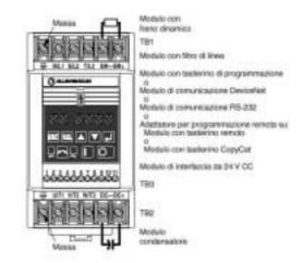
Figure 29: frontal view of the inverter .
