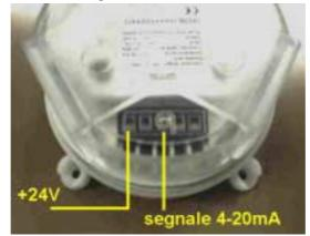
Figure 24: terminal board of the differential pressure switch.
