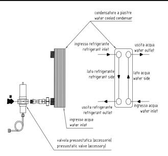
If the feeding water comes from a well or a river, two filters shall be installed in parallel, one of them as backup, with features conforming to the type of water used, to prevent the condenser from getting clogged due to impurities in the water.
