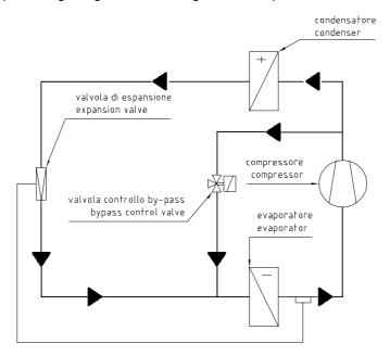
This system allows a modulation of the cooling capacity between 5% and 100% of the nominal one, therefore also with a great reduction of the absorbed power at the same time.
