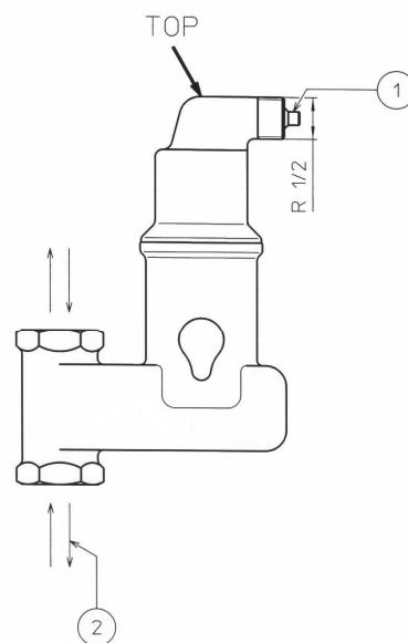
venting valve, remove obstacles for air release from the venting valve.
