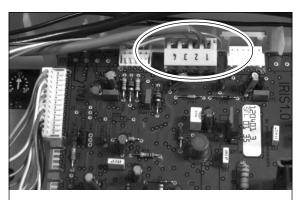
Connect the probe cable (15 m) to the main card to the right of the 5-pin flat cable connector.
