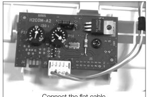
Connect the flat cable (3-core connector) to the probe card
