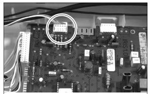
On the main card, replace the flat cable already installed with the one from the kit (5-pin connector) (Scrap the old one)
