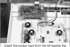
Insert the probe card from the kit beside the interface card, using the screw
