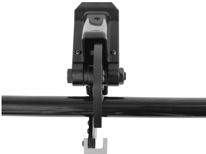
Figure 2 – Cutting Edge Lined Up With Wire Mark
