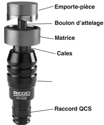
Figure 1 – Tête de poinçonnage PH-60B
