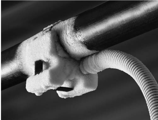
Figure 9 – Freeze Head Frozen to Pipe
