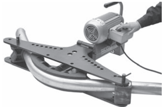
Figure 14 – Operating the Electric Bender
