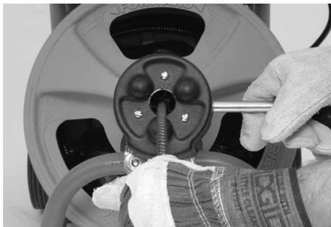
Figure 14 – AUTOFEED in Retrieve Position
