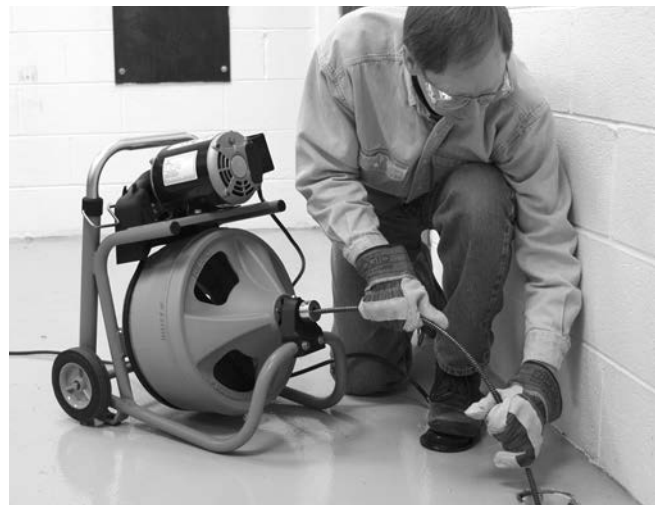
Figure 12 – In Operating Position, Manually Feeding Cable
