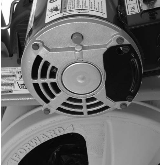
Figure 8 – Drum Rotation Direction Arrows
