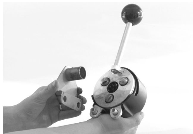
Figure 3 – Placing Mounting Bracket Into AUTOFEED
