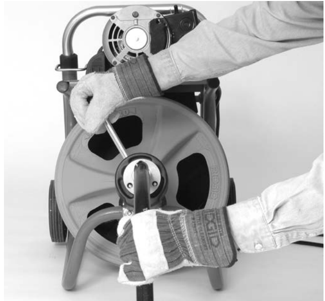
Figure 15 – Using Machine with Guide Hose
