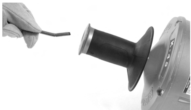
Figure 17 – Loading Cable Without Changing Inner Drum
