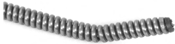
Figure 15 – Bend At Cable End
