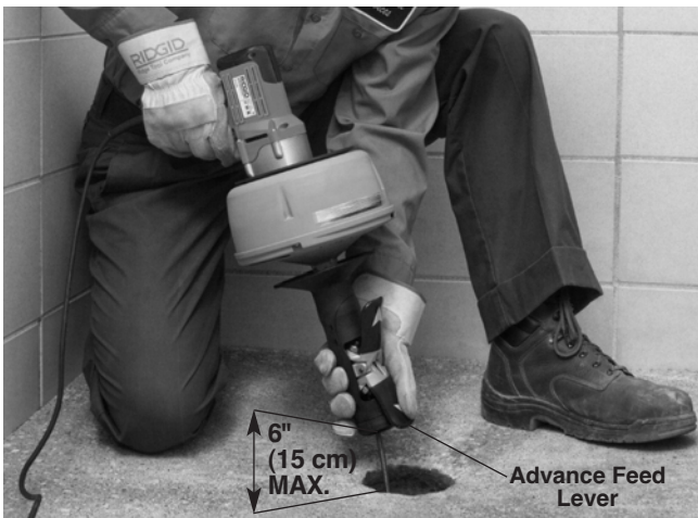
Figure 10 – Feeding Cable With AUTOFEED
