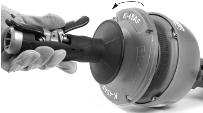
Figure 14 – Twist Drum Apart
