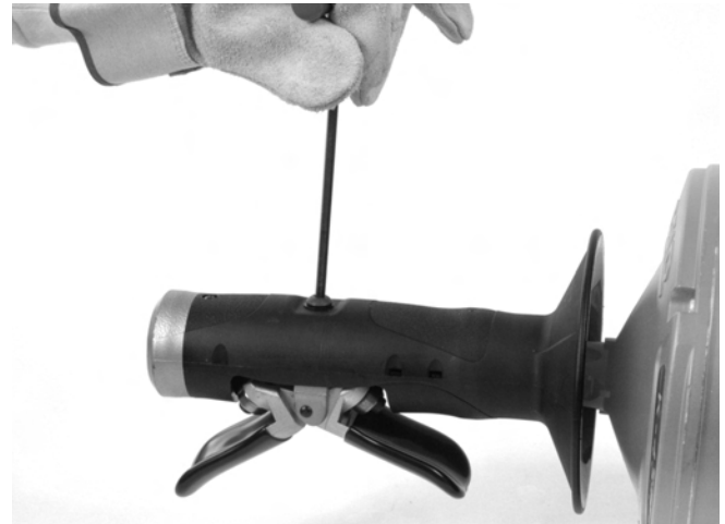
Figure 12A – Removing AUTOFEED Screw
