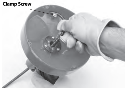
Figure 9 – Installing Cable End Into Holder
