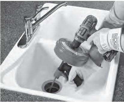
Figure 8A – Power-Spin Powered By Battery Drill
