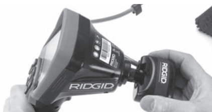
Figur 19 – Kameraets tilkopplingsplugg installert
