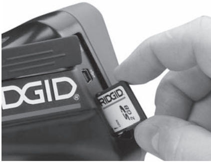
Figure 10 - Inserting the SD Card
