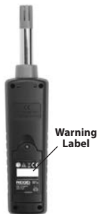
Figure 2 – Back of micro HM-100 Temperature Humidity Meter
