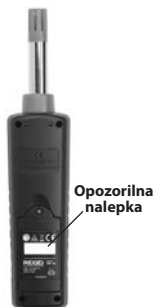
Slika 2 – Zadnja stran merilnika temperature in vlage micro HM-100
