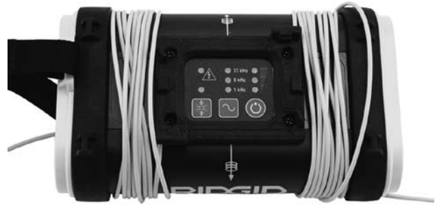
Figure 11: ST-305 in Inductive Mode at 33 kHz
