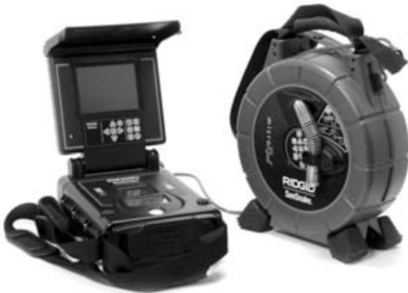
Figure 18 – microReel System Connected to SeeSnake® DVD Pak CCU
