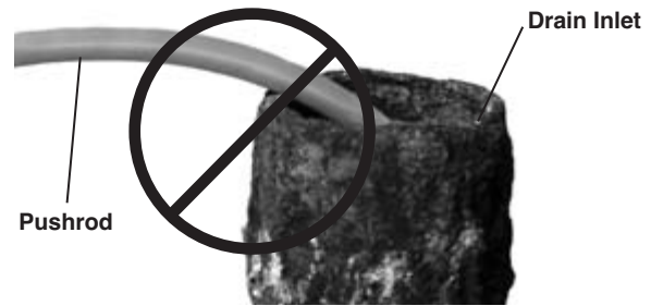
Figure 23 – Avoid Pulling At Sharp Angles
