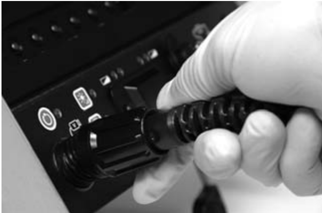
Figure 17 – Connecting To A SeeSnake CCU
