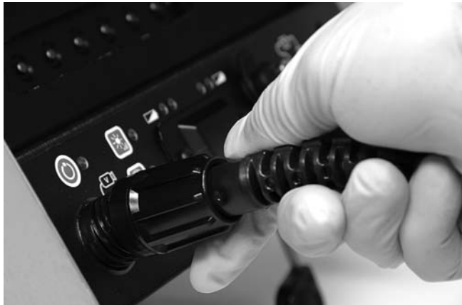
Figure 13 – Connecting To A SeeSnake CCU
