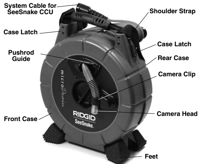
Figure 1 – Front View (SeeSnake Configuration)
