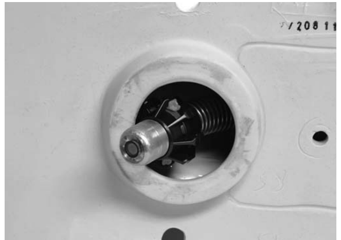
Figure 21 – Camera Head with Ball Guide in Turn
