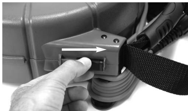
Figura 4 – Deblocarea carcasei bobinei microDrain.
