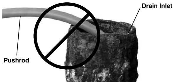
Figure 18 – Avoid Pulling At Sharp Angles
