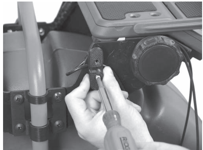
Figure 16 – Mounting the Cord-Wrap (Note USB Cable captured under Cord-Wrap)
