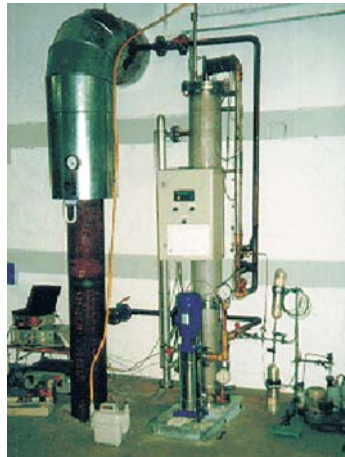
Figure 2: Nitrogen reduction using 'servitec' partial flow degassing in a test system of the Halle energy utility
