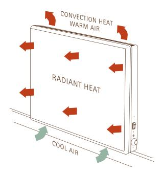
Just like the sun, radiant heat is multi-directional, and works on the principle of warming surfaces and objects within a room. Radiant heat is universally regarded as a very efficient, healthy and comfortable method of heating.
