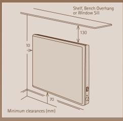
The recommended height off the floor is a minimum of 70mm. The sides of the panel heater can be installed within 10mm of a corner or furniture located against a wall. Directly under windows is an ideal location.
