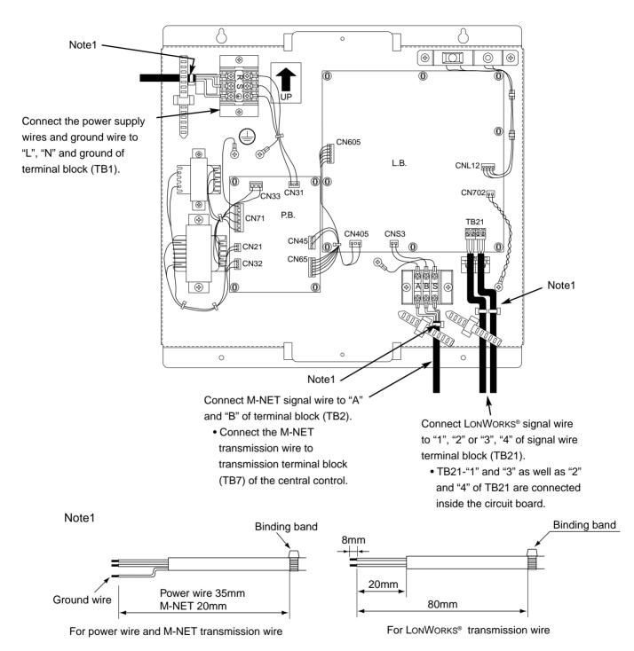
Attach the appended binding band to the power wire and transmission wire, and fasten it, positioning the area at inner side than the wire clamp.
