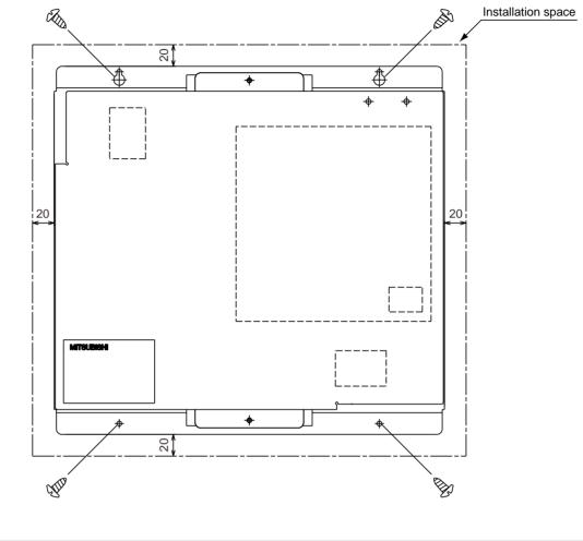
This unit does not have a water-resistant design. Always install the unit indoors or inside a control panel.
