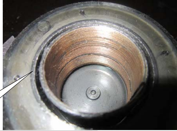
The scroll plate is worn.
