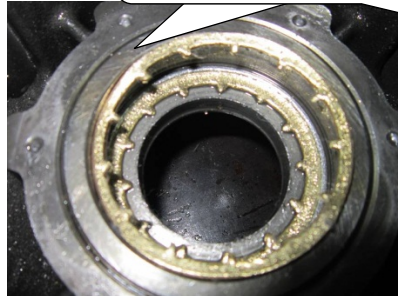
The filter is blocked by impurity, the suction of the compressor will be abnormal
