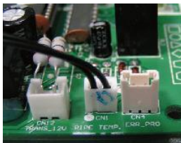
Compressor current protection
