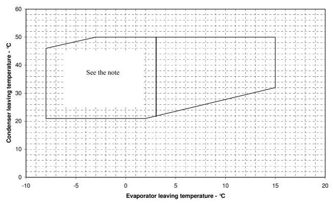
Note: the use of glycol is necessary for evaporator leaving water temperature below +3 ℃.
