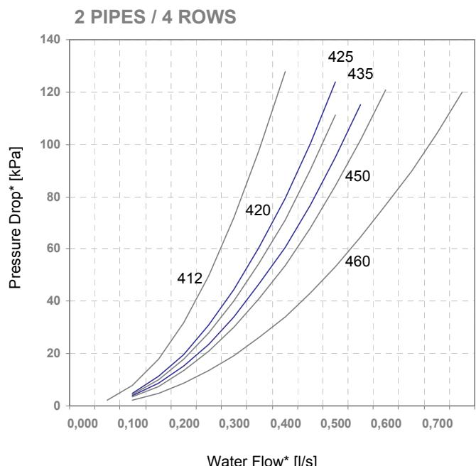
\*The pressure drop is for coil only and excludes water connections and valves.
