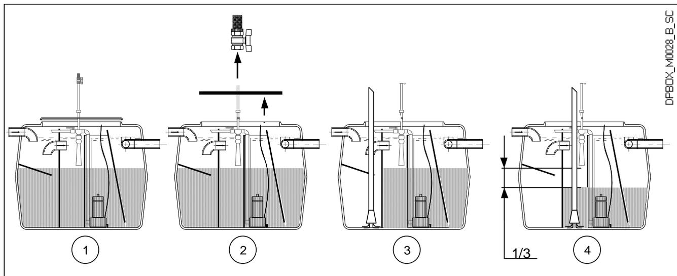
10.9.2 Depurbox Maxi and Duo (Imhoff tank) – Sludge removal
