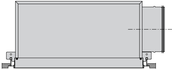
Plenum box type H including mounting bracket type PBB
