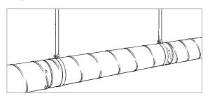
Mount the hangers in a straight line and as close to every joint as possible. Fix with an extra screw when needed for extra stability.
