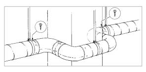
In situations where the mounting must be locked, e.g. when a bend is mounted to a duct and it twists downwards the floor. Mount the first hanger and mount the bend, then lock the joint with a screw or blind rivet.
