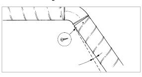
Mount the next piece of duct at an angle, but make sure that the rubber sealant is not visible. Put screws or blind rivets where the notches have not clicked in position.
