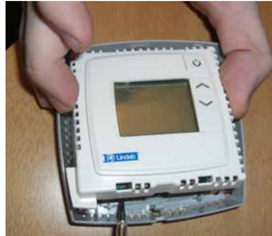
2. Remove the front including the circuit board
