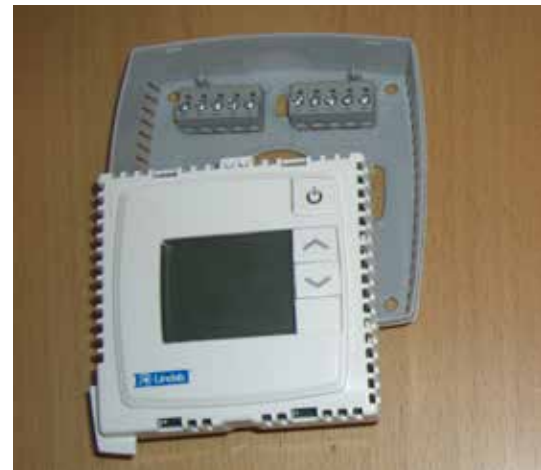
4. Remount in inverse arrangement when the plinths are connected. Notice that the front and bottom plate only can be fitted to each other in one way. See mark "UP".
