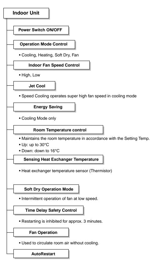
• The power comes on again after a power failure.
