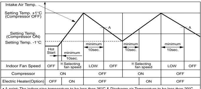
• A point: The indoor pipe temperature to be less then 35°C & Discharge air Temperature to be less than 29°C. The indoor fan operates for minimum 10sec. even if falls lower than 34°C.
