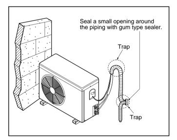
Drain water treatment of outdoor Unit(Heat Pump Only)
