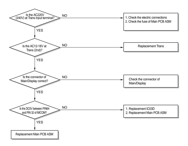
4) Timer control does not operate. — Replacement MICOM
