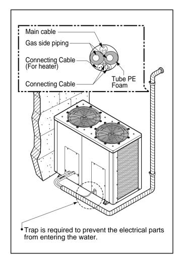
In case of the outdoor unit is installed upper position of the indoor unit.
