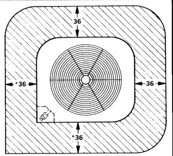
NOTE — 48 inch clearance required on top of unit.
