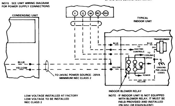
CONDENSING UNIT FIELD WIRING DIAGRAM
