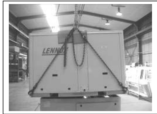
Use protection between the machine and the lifting rings
