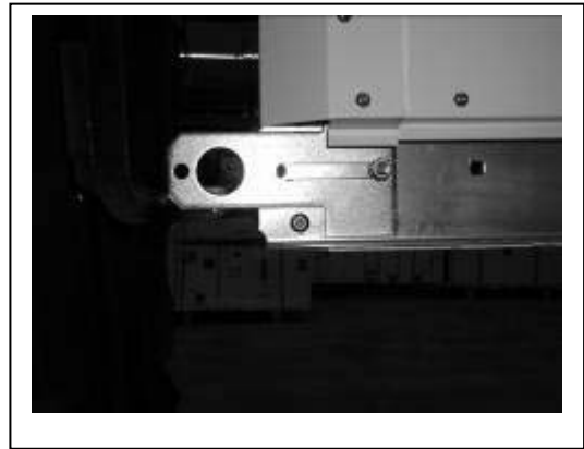
Lifting lugs After unfixing the screw ref A, move the 4 lifting lugs out of the frame then fix it again
