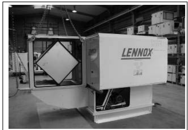
Bring the module on the support. Check the good shape of the 20 x 10 black gaskets.
