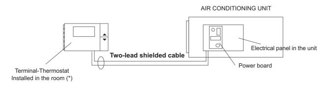
(\*)If remote sensor is requested as an option, the terminal-thermostat can be installed in a different place from the room to be conditioned.
