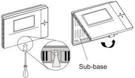
3° To fasten the rear part of the box to the wall, place the hole in the centre of the box over the cables for the control of the instrument which come out of the wall. The placement of the mounting holes has been designed to allow the instrument to be fixed onto a box conforming to standards CEI.431 - IEC 670 (100x600). If this is not available, use the mounting holes on the shell as a guide for drilling holes into the wall and then use the screw and plug kit supplied.
