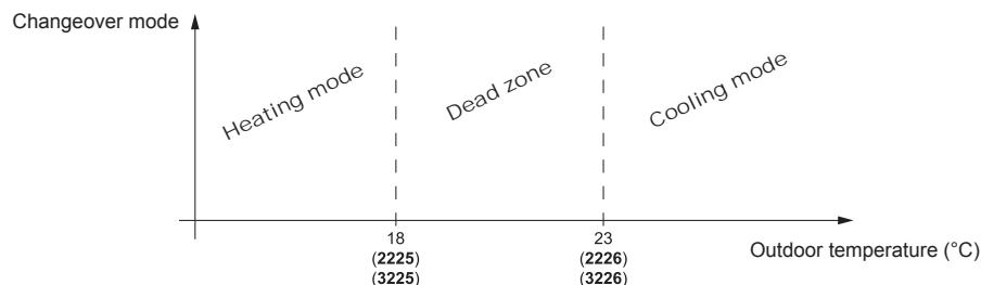
If the outside temperature is below the setting value (2225) or (3225), the unit will operate as a heat pump.
