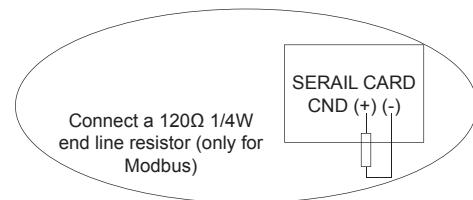
**!** The connection must be carried out by the following cable: length up to 1000 m: LiYCY-P (0.34 mm<sup>2</sup>), 2 pairs with general shield.
