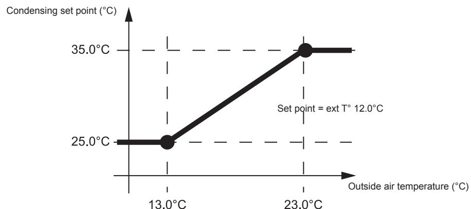
Note: this functionality can be disabled if the selected setting (**3546**) is different from the factory value. In this case the condensing set point is the new selected value.
