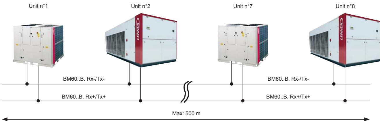
The pLAN bus is connected to CLIMATIC™ 60 on the J8 connector of board BM60. A star connection is not recommended. For an optimum operation it is advised to connect a maximum of two cables per unit.
