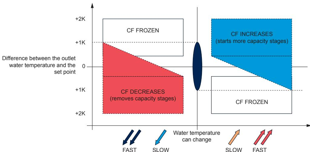
In order to anticipate, the reference point is recalculated each time the difference between air temperature and set point reaches a minimum or a maximum.
