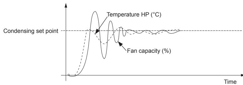
In order to optimise the performance of the unit, the condensing temperature is set according to outside air temperature and tries to maintain a delta of 12°C (only for unit with electronic expansion valve).
