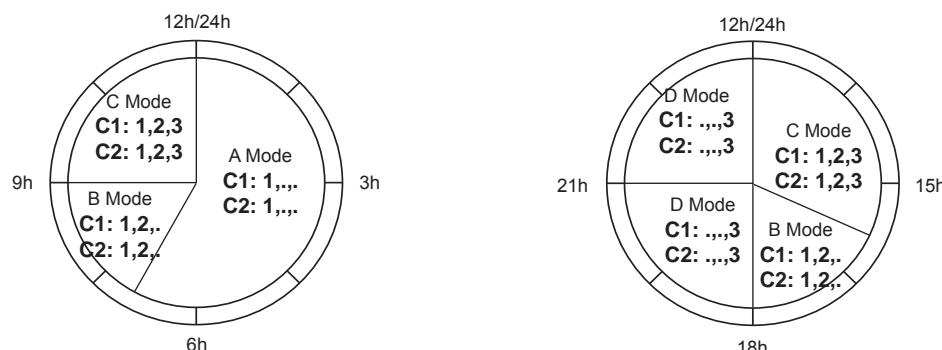
Moreover, the circuit priority can be specified (for units with 2 circuits)
