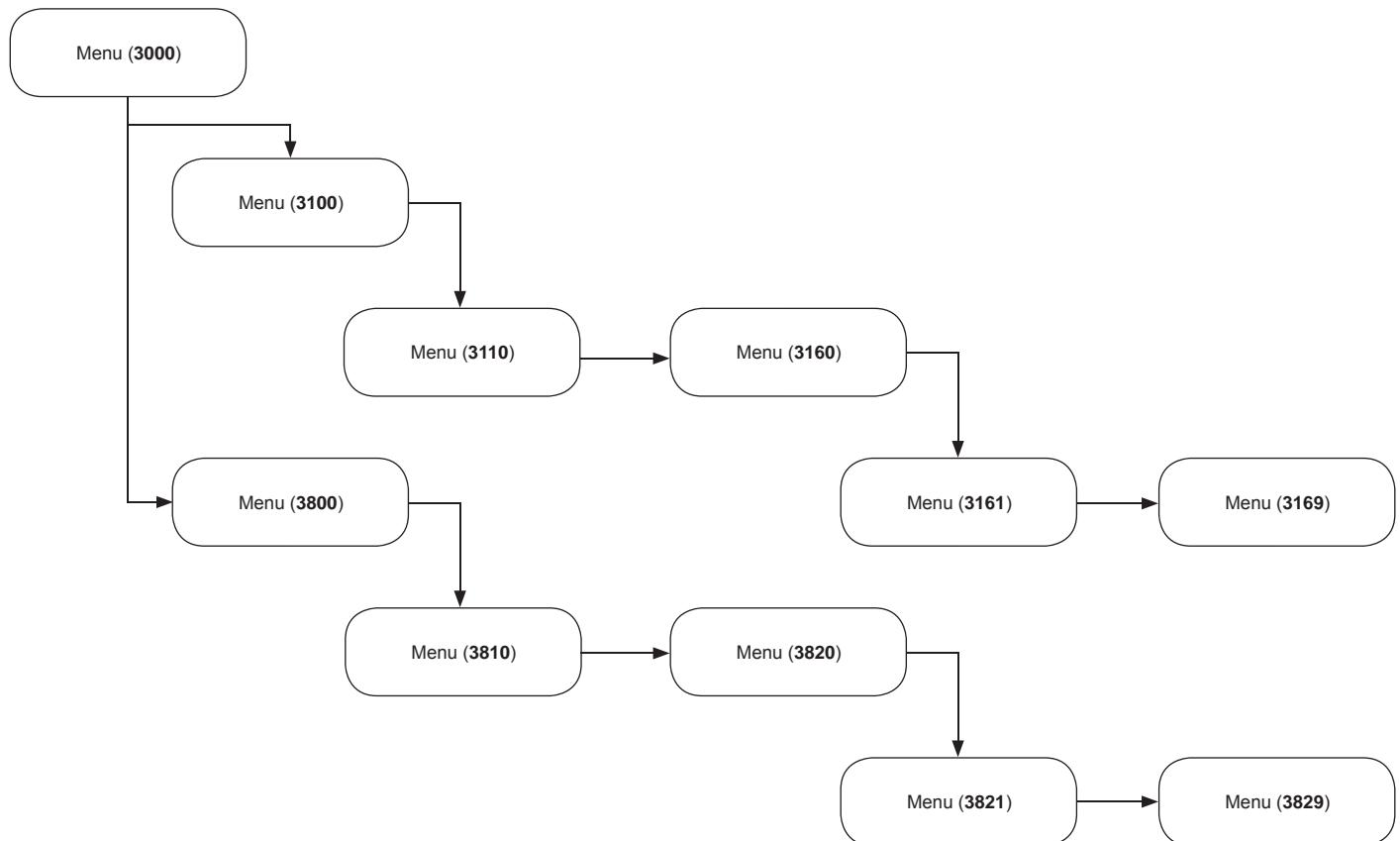
The “↓” and “↑” keys are used to move the cursor on the desired item. Then use the “←” key to enter in the selected submenu. To escape a menu use "ESC" the key.
