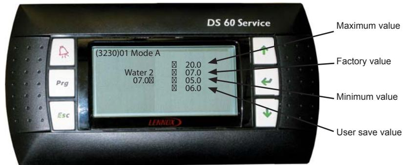
☞ to quickly increment or decrement the setting, hold the “↓” or “↑” keys during few time.
