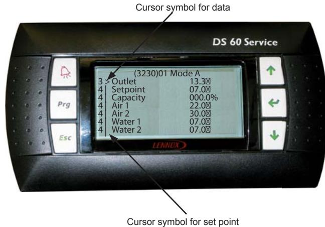
To modify a setting, move the cursor on the desired item and press the “←” key. A new screen displays information concerning this set point. To modify it, use the “↓” and “↑” keys and validate by pressing the “←” key. If the setting is customizable according to the schedule mode, press the “PRG” key to select different value for the A, B, C& D mode.
