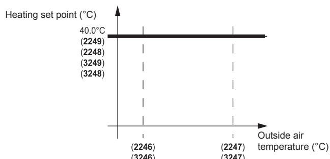
The cooling and heating set points can be pre-specified according to the scheduling and can take different mode for each schedule mode (Night, Day, Day A, Day B, and BMS)
