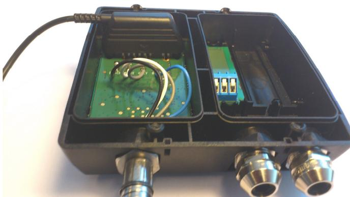
Figure 44. Location of the four-pole plug in ULTRAFLOW® 54 DN150...250.
