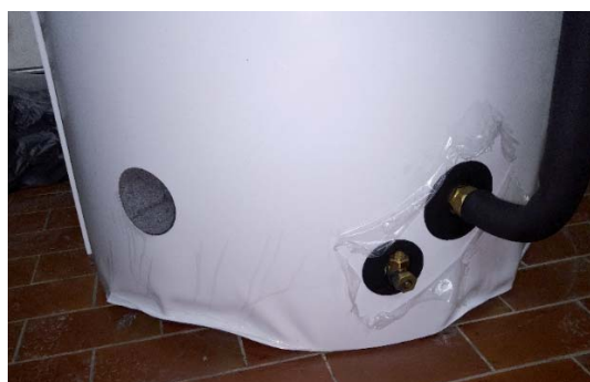
pic.: Damaged insulation caused by improper storage.
