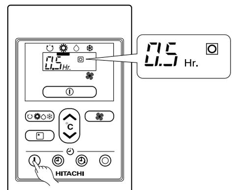
■ Operation will start for setting temperature at setting time (The starting time may different depend on the room temperature and set temperature).
