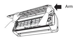
When the front panel is fully opened with both hands, push the right arm to the inside to release it, and while closing the front panel slightly, put it out forward.
