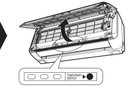
Do not hold the moveable panel when the front panel is in either opened/closed position.
