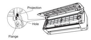
Move the projections of the left and right arms into the Flanges in the unit and securely insert them into the holes.
