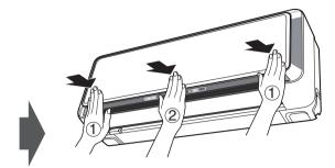
Initially press the left and the right sides of the front panel and finally press the central portion until you hear a clicking sound.
