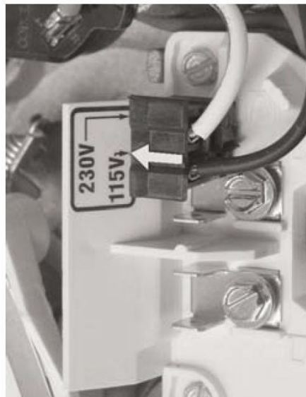
Voltage change plug set for 115 volts Fig 3.9.2
