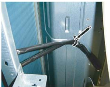
Loose the clamp, and remove the lead wires.
