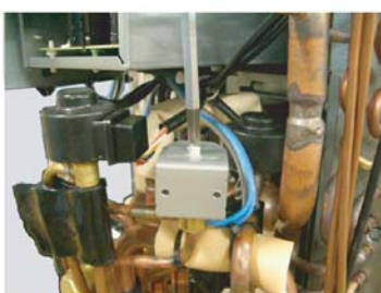
Remove the mounting screw.
