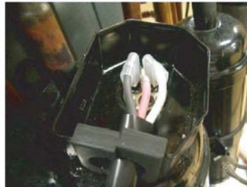
Remove the connectors. [ R : RED, C(T) : BLACK, S(W) : WHITE ]
