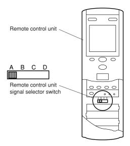
Confirm the remote control unit signal selector switch selection and printed circuit board setting. If these are not confirmed, the remote control unit cannot be operated for the air conditioner.
