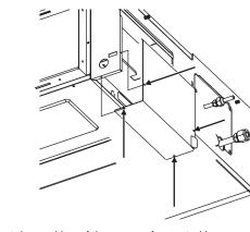
Adjust the position of the screws for control box cover according to the installation.
