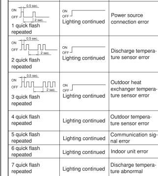
When the fault is cleared, the LED lamp goes off. However, for discharge pipe temperature abnormal and high pressure abnormal, the LED lamp lights continuously for 24 hours, as long as the power is not turned off.
