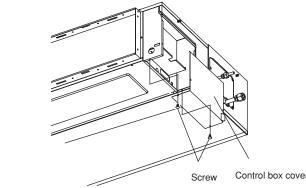
(2) After wiring is complete, secure the remote controller cord,
