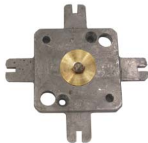
10- Install the LPG aluminium front part of the firing head cod. BFT12119 (Natural Gas cod. BFT12116) and the LPG (Natural gas) nozzle. The notch of the nozzle must be in the correct position.
