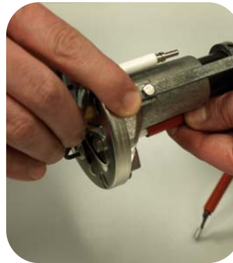
7-Reassemble the cable of ignition and ionization.
