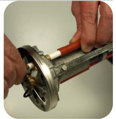
4-Remove the cables of ignition and ionization.
