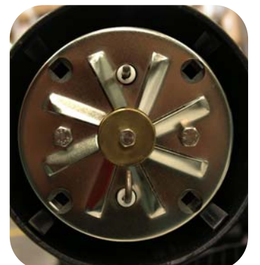
12- Reassemble the blast tube in the burner.
